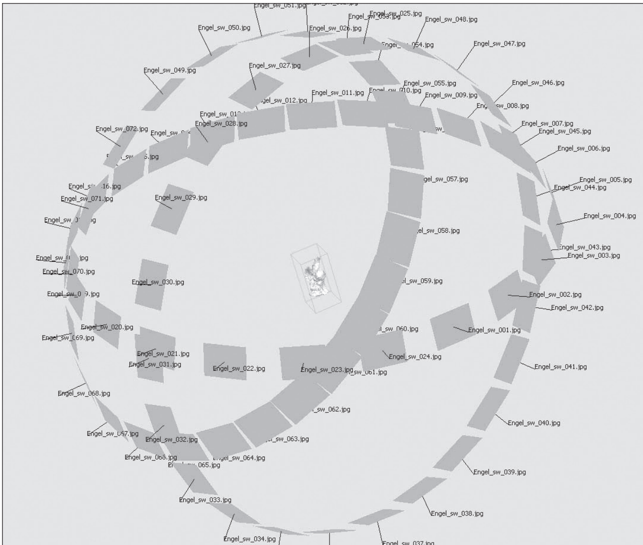
3. Structure from Motion (SfM) as used by Agisoft Photoscan photogrammetry software.
